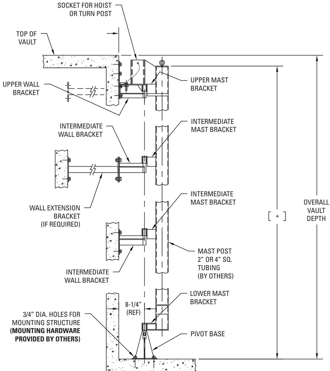
\* USF FABRICATION RECOMMENDS USING ONE (1) INTERMEDIATE MAST BRACKET AND WALL BRACKET AT 10 FT. INTERVALS
