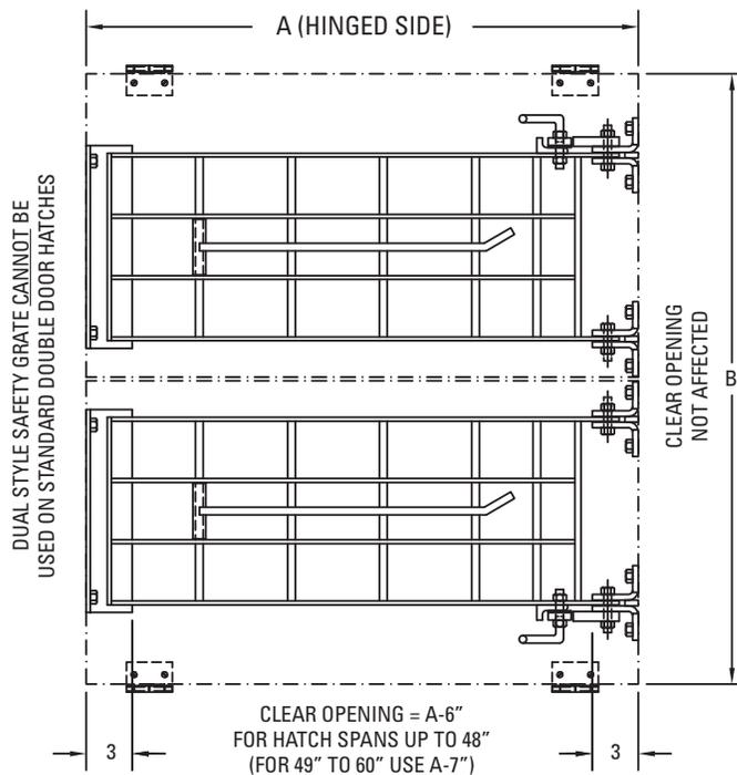
**STANDARD DOUBLE DOOR HATCH (HINGED OPPOSITE SIDES) WITH STANDARD SAFETY GRATE**
