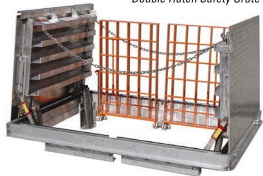
For large openings, USF Fabrication makes a dual safety grate that hinges on opposite sides of the hatch frame and double safety grate that hinges on same side of the hatch frame. These configurations can place a barrier on three sides of the hatch's opening. A safety chain can be employed to block the fourth side of the opening.
